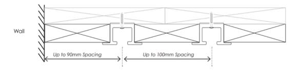
Using the same basic principles to determine the width as for standard tracks and rods as outlined above, measure exactly from where you would like the track to start and finish. **This is your overall track width.**
