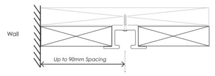
A straight double track system should be measured and fitted 60-90mm from the wall for the first (rear) track and 90-100mm from the first track to the second (front) track (centre to centre - see diagram below).
