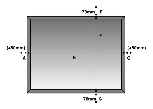
A (50mm) + B (width of architrave to outside edges) + C (50mm) = Overall width
