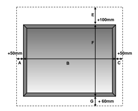
**A** (50mm) + **B** (Width of architrave to outside edges) + **C** (50mm) = Finished width **E** (100mm) + **F** (Height of architrave to outside edges) + **G** (60mm) = Finished Drop
